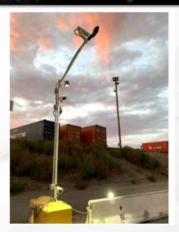
enVision In Lane OCR portals to image and ID containers, chassis, & truck license plate Options for damage inspection, seal detection
